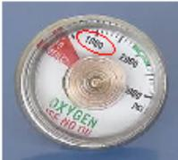
At 1000 PSI or less, switch for a new O<sub>2</sub> tank
