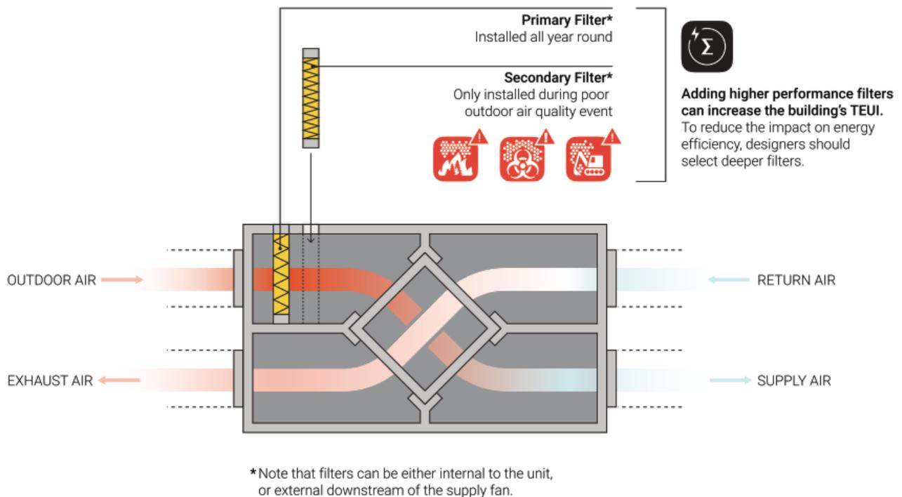
Figure 20: Filtration guidance for energy recovery ventilators (BC Housing, 2019).
