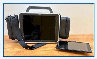
The Monitor by Laerdal is a simulated patient monitor system that can be used to control and project vital signs using iPads. This can help add fidelity to scenarios with low fidelity manikins.
