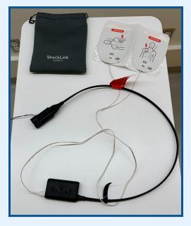
ShockLink allows users to use live defibrillators on Laerdal manikins. The device is connected to a defibrillator and a set of specially designed pads. The ShockLink device absorbs the live energy from the defibrillator while communicating the necessary information to the instructor's and learners' devices.
