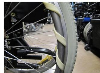
Ensure adequate friction. Use of mitts, gloves, dycem, or surgical tubing all impact a wheelers control over the chair. Also consider if the hand rim is suitable friction coated handrims, rims with lugs, and rims with different cross sections may make a significant difference
