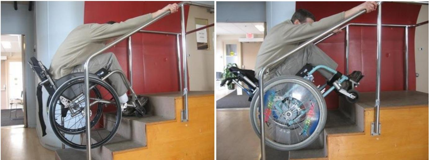
Note the difference in angulation at the same point due to the different chair geometries
