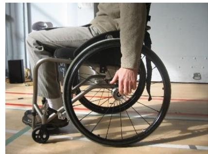
Camber and offset can be adjusted to make holding the push rim more comfortable. Sometimes armrest pads interfere with the wheelers ability to wheel and can be removed temporarily or reversed to allow longer contact. Generally 3-6 degrees of camber is comfortable. Having the tops of the wheels positioned directly below the shoulders and the middle finger resting over the axles when the arms are hanging is a good starting position.
