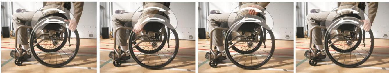
Generally SLOP is a little more efficient than the Arc style. There is no braking effect from having the hands in contact with the rim during recovery. However, the limited time spent in contact with the rim during each
