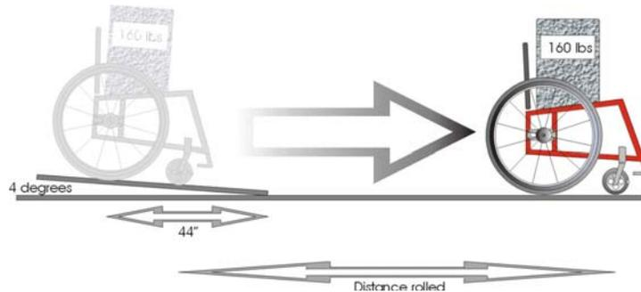
The distance rolled in this type of test is inversely proportional to the effort required to wheel the chair.
