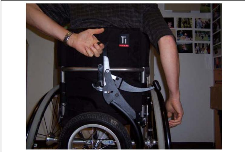
Setting up the perch for the free wheel which clamps to the rear rigidizer bar when not in use is simple enough but I suggest taking time to experiment with the angle the “U” shaped post is fixed at. It took me 15 to 20 seconds of fiddling each time I wanted to clamp the free wheel to the post. After I adjusted it so that the clamping shim was parallel to the straight surface when the free wheel hung from my finger it took less than 5 seconds and no fiddling.
